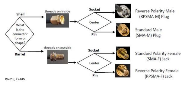
The source of confusion lies in the fact the gender of the connector is commonly determined by the shape of the center conductor. A male connector (plug) is a pin that sticks up from the center of the connector's insulated surface. A female connector (jack) is a socket recessed into or below the center of the connector's insulated surface.
