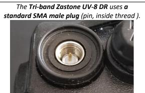
Currently the following Dual Band antennas in the GECO inventory are intended to be directly attached to the radios. All these antennas have standard SMA female jacks on their bases. This first set of antennas are primarily allocated for use with the Bao Feng radios.
