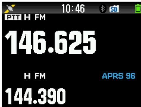
As in the third image, when TUNE is selected, the radio automatically tunes to the frequency of the second band (non-data band).
